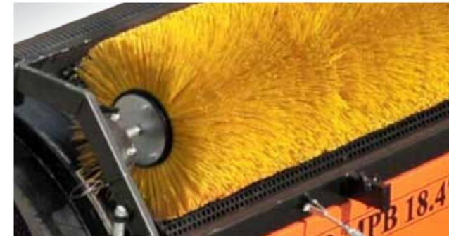
Hydraulically raised and lowered trommel cleaning brush
