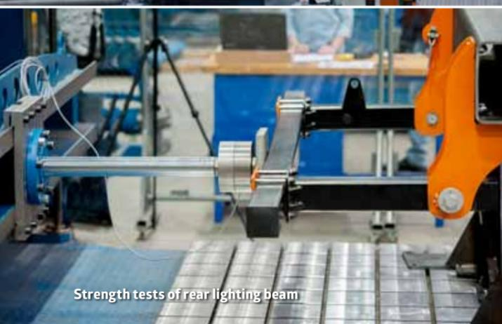
Strength tests of rear lighting beam
