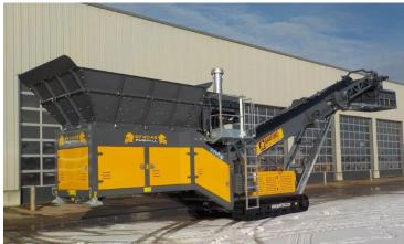
Tracked Pugmill - Hyd Adjustable Mixer Box, Full PLC System, Cement Weigh Hopper, 400LTR Fuel Tank, Brevini Gearbox, Eaton Motors.
