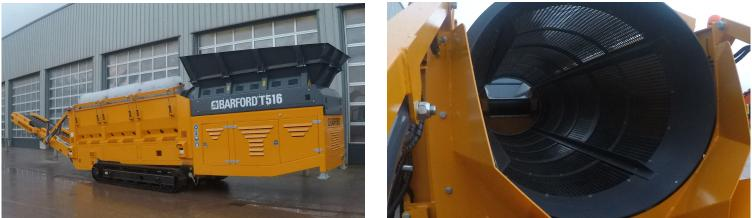
5'x16' Drum, Variable screening angle, Hopper capacity: 3.8M<sup>3</sup>, Feeder belt width 950mm, Side conveyor belt width 650mm, Transfer conveyor belt width 1050mm, Oversize conveyor belt width 950mm, chevron belt, Power unit: CAT 4.4 74KW Engine, Tracks: 2.9M tracks \* 300mm shoes, Remote Control Movement
