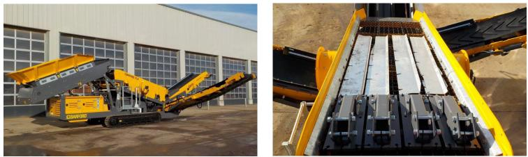
Barford SR124 Heavy Duty 3 Way Split Screen, 12' x 4'2" (3.66m x 1.28m) Screenbox, CAT 4.4 (56kw/75hp), 40" Heavy Feeder Belt, 40" Heavy Chevron Overs Belt, Impact System in Hopper, 42" Fines Collection Conveyor, Telescopic Extending Side Conveyors.
