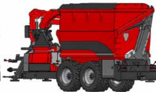
20/25 m³ telescopic to 4.55m tipping height
