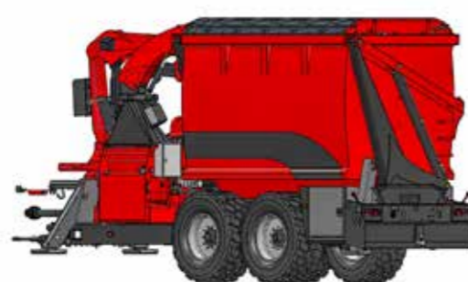
20 m³ right side tipping 25 m³ left side tipping (covers open)
