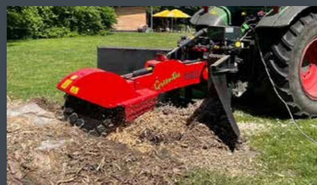
Drive line runs fully protected through heart of machine
