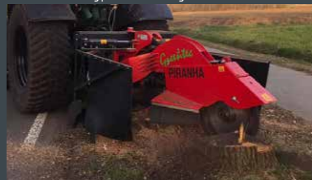
All-round shielding: minimises flying debris
