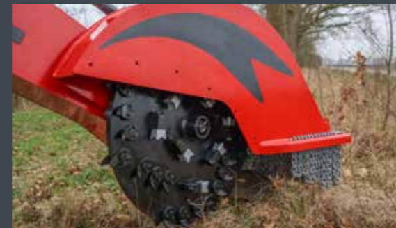
Optional with 8 cutting teeth, to grind away bushes
