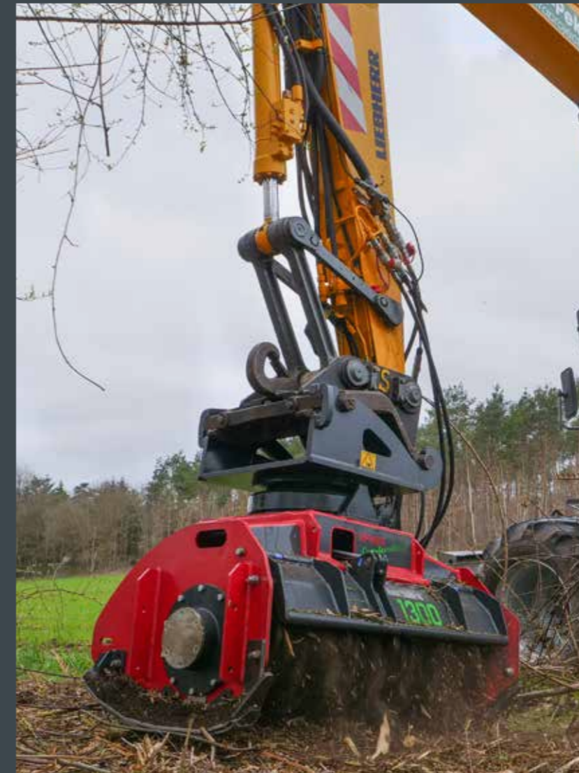
Adjustable Hardox anvils (rotatable)
