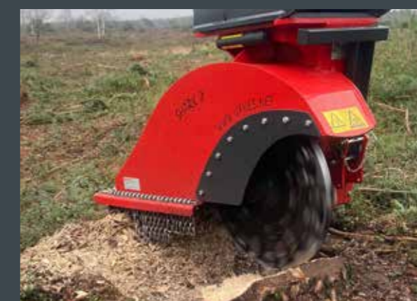
All-round shielding to minimise flying debris
