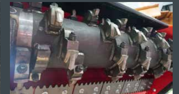
Adjustable Hardox anvils (rotatable)
