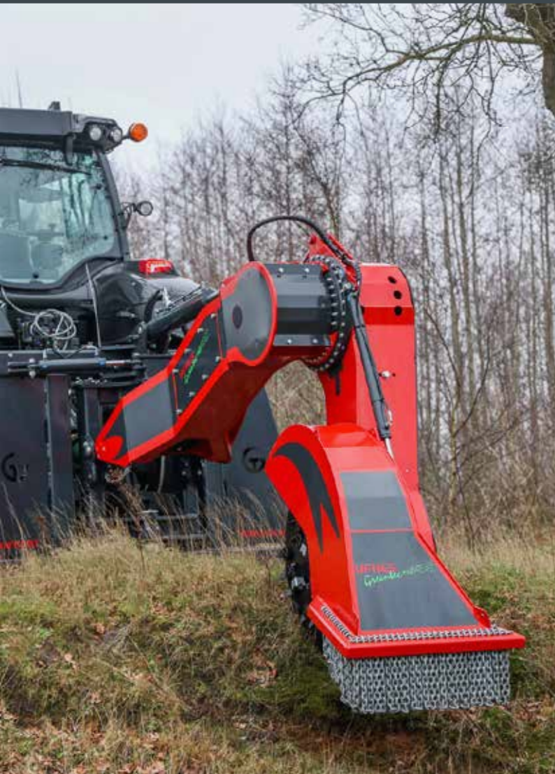
Optional with 8 cutting teeth, to grind away bushes
