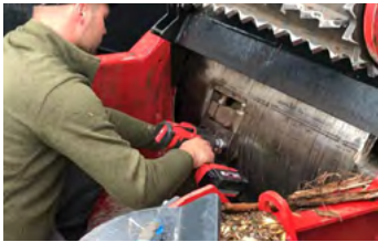
Knives easy accessible when the infeed rollers are hydraulically positioned above the machine
