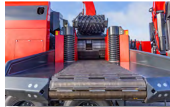
Continuous infeed chain to below the top roller(s) optionally
